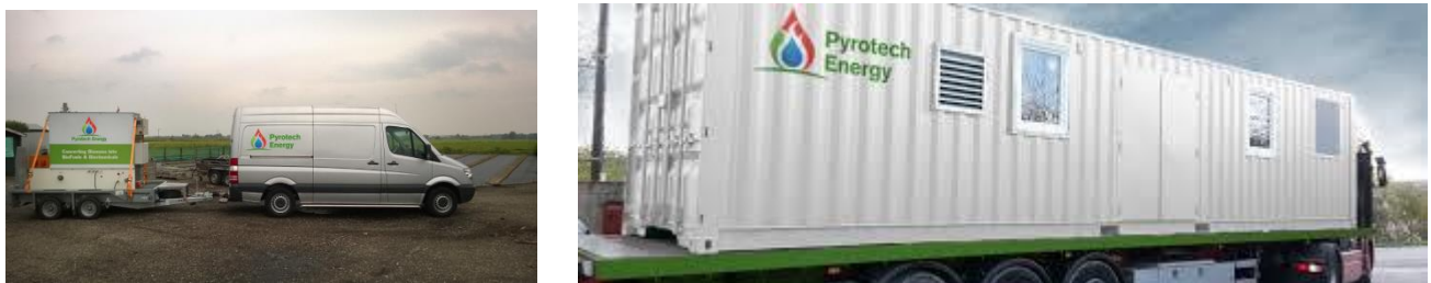
Figure 2. The mobile pyrolyser with 2 and 10 tonnes per day feeding capabilities
